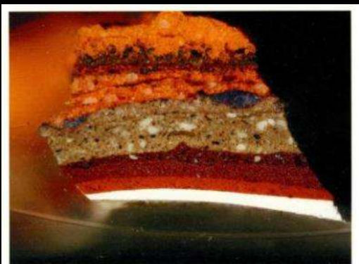
Cross section from the 'arm' of the Maori House viewed under the microscope (x10) with reflected light showing thirteen paint layers.
