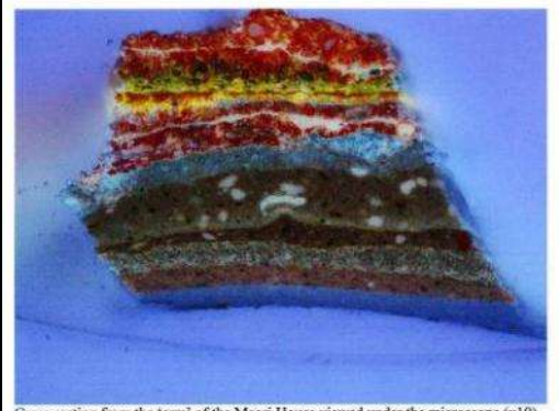
Cross section from the 'arm' of the Maori House viewed under the microscope (x10) with light showing the fluorescence of the thirteen paint layers.
